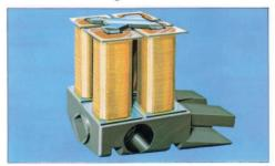
The cylinder is made of carbon fiber reinforced plastics that is three times physically stronger than the conventionally used resin (ABS). This has eliminated unnecessary resonance, causing a Clearer sound. Magnetic shield casing For realisation of a high SN ratio, super permalloy, that is outstanding in magnetic shield characteristics, has been adopted.
